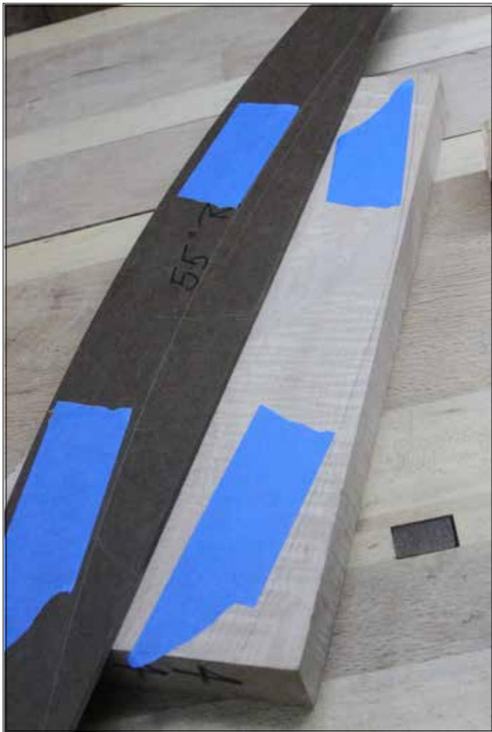
Speaking of templates, Mark makes his by gluing a printed paper template to a bit of 1/2" MDF, then roughs the outline on the bandsaw, followed by careful sanding to fair the curves. It's important to keep the edges square, so Mark uses a sanding block with a fence to keep the block perpendicular to the surface. The problem is, after a bit of sanding that area of the
