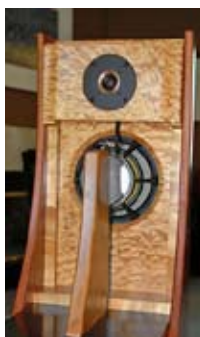
The rear of the Orion speaker. There is no back. The sound comes out from both the front and back.
